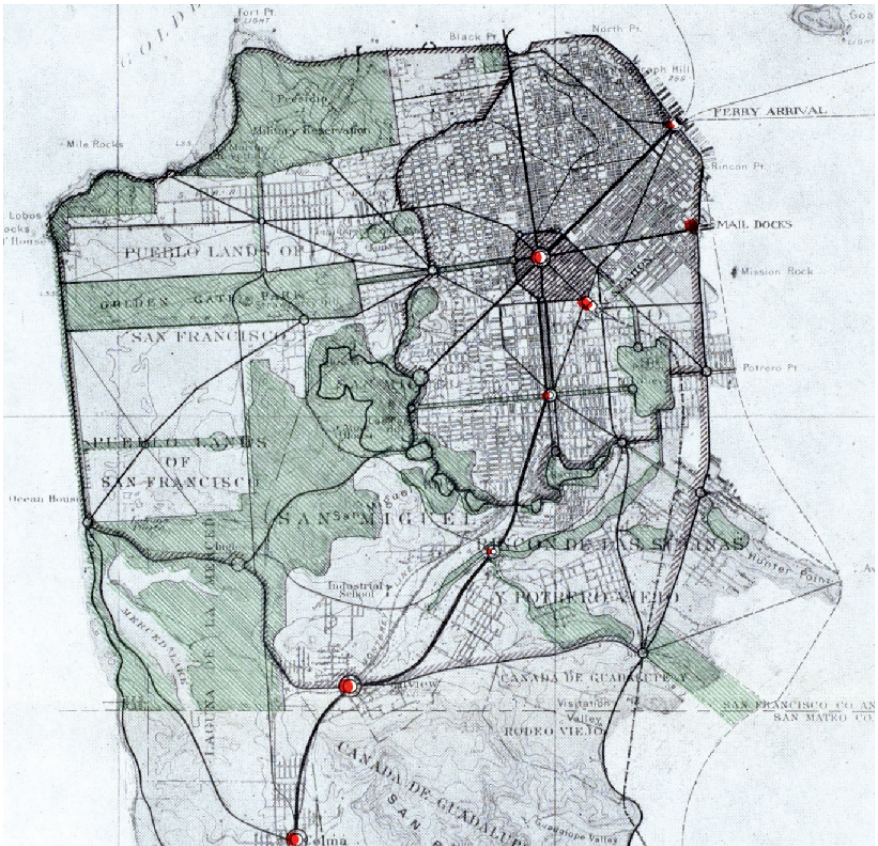
D. H. BURNHAM, DETAIL OF THE PLAN OF SAN FRANCISCO SHOWING THE SYSTEM OF CIRCUITS AND RADIAL ARTERIES, FROM THE REPORT OF 1905.
