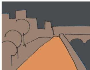
c) *The Background View Analysis* disregards the sky & river components of the image and takes into account the pathway and the background components. The absence of the sky and river elements from the image's luminance measures results in a photometrically more accurate representation of the lit scene.
