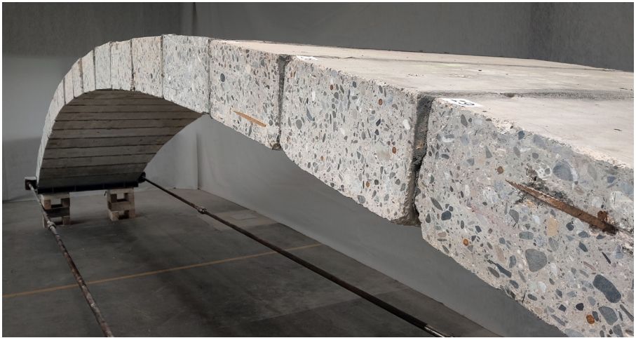
Re:create, an arch made of reused concrete blocks. https://doi.org/10.1016/j.istruc.2022.07.012 © SXL, EPFL
