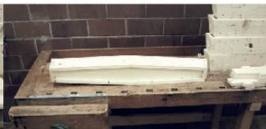
Physical prototype test: an arch formed of hexagonal box components.
